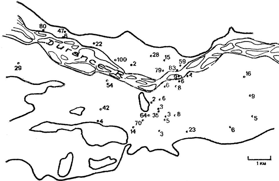
FIG. 15 - VALEURS DE LA TRANSMISSIVITE (EN  $10^{-2} m^2/s$ ) MESUREES
