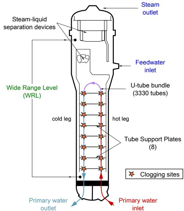
**Fig. 1:** Westinghouse type 51 SG principal elements
